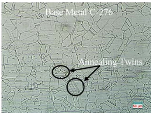
Fig.3 Microstructure of alloy C-276 in as received condition.
