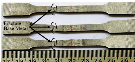
Fig. 6 Photographs of tensile failure specimens
