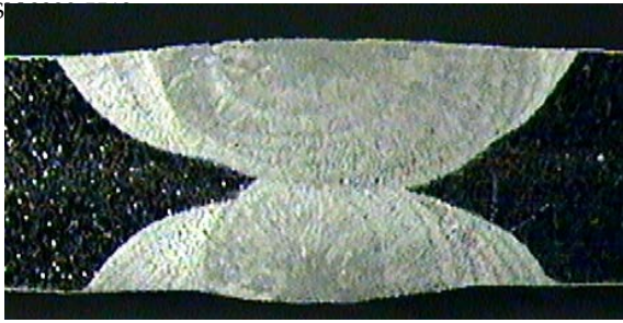
Fig. 2 Macrostructure of Autogenous PCGTA Weld joint Magnification: 1.25
